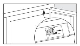
■ Unscrew the lamp and replace it with a new one.
